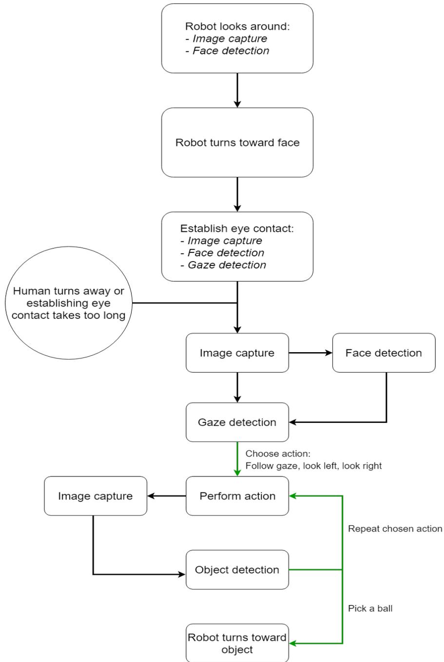
Figure 1: The final pipeline. The italic words are the subcomponents that the robot performs continuously while within the main component. The green arrows and box indicate that at those points, the robot has to make a decision.
